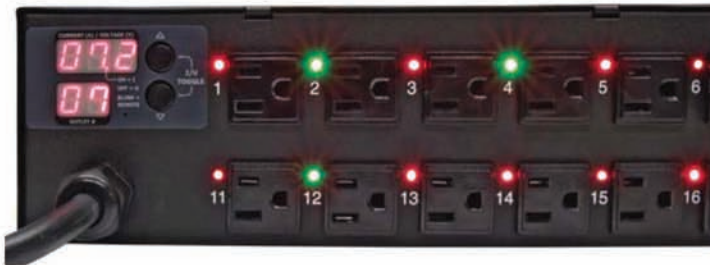
Rear of 2U PDU showing current draw for outlet #7. Red LEDs show outlets that are switched on. Green LEDs show outlets that are switched off.
